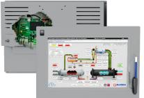
The MCS-NitroMag-15.4 is a control system containing a Capacitive Touchscreen, and a MCS-NitroMag-N controller. It includes a processor, memory, eMMC Flash, and supporting power circuitry. The Broadcom quad-core processor on the MCS-NitroMag-N delivers a blazing speed of 1.5GHz.
